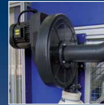
Fig.: Reinforced grinding dust extraction unit
