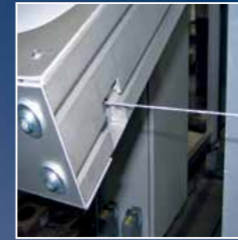
Fig.: Exit side of the cutting wire
